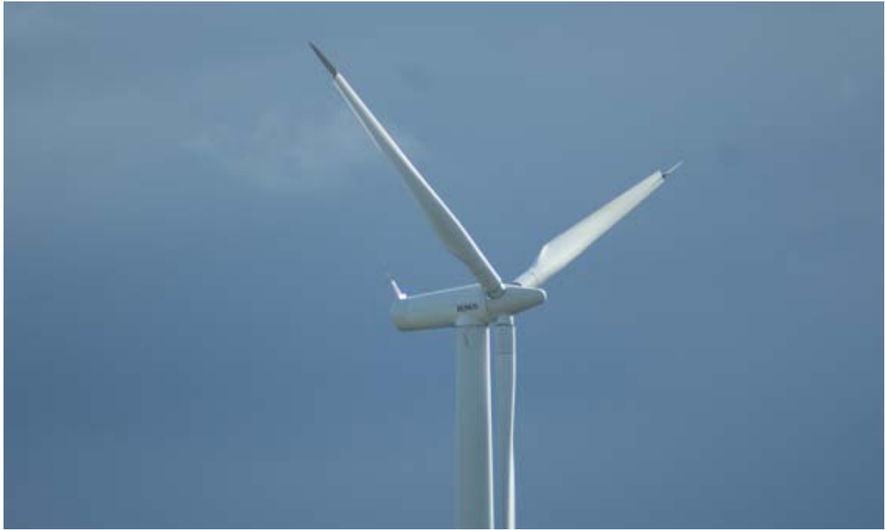
FIGURE 33: WIND TURBINE WITH STALL CONTROL AND WITH RELEASED TIP-BRAKES.
