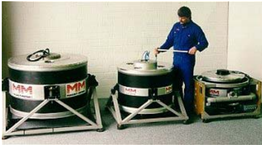
Figure 8 Three flywheel energy storages. The peak specifications are 80 MJ / 5 MW for the biggest and 80 MJ / 2.5 MW for the medium sized. The smallest is not known at the time of writing.
