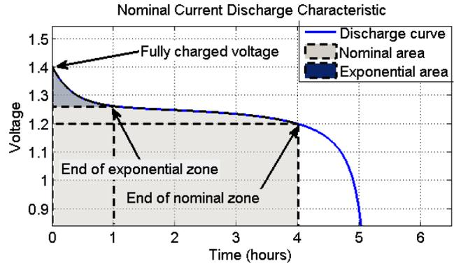
Fig. 2. Typical discharge curve
