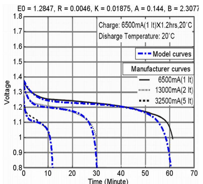
Fig. 8. Nickel-Metal-Hydrid battery 1.2V 6.5Ah
