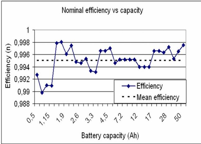
Fig. 4. Efficiency at nominal current vs battery capacity
