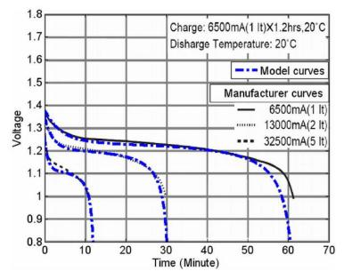
*Calculate the battery capacity with different discharging currents. Which case gives a bigger capacity? Why?*
