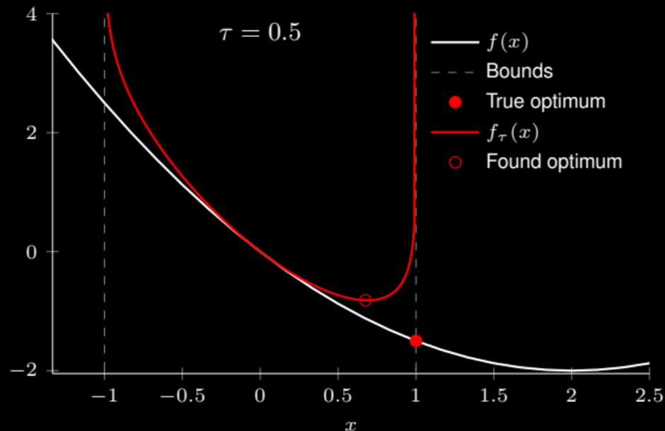
Figure 30: Illustration of the interior point barrier method.
