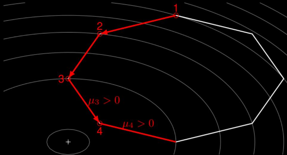
**Figure 25:** Illustration of active set method with two decision variables and initialised with two active constraints. The feasible region is within the octagon, the contour lines indicate the level sets of the cost function, the plus indicates the unconstrained optimum and the filled circle indicates the optimal solution.
