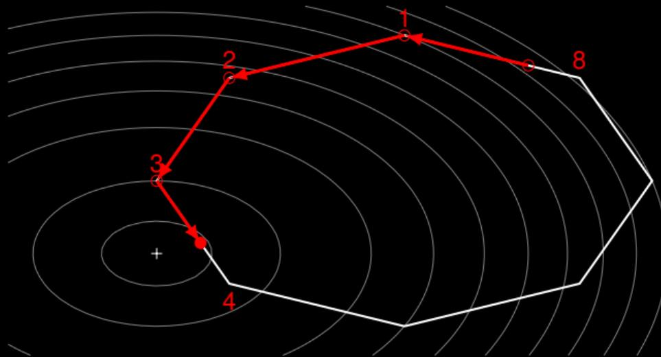
**Figure 28:** Illustration of active set method with two decision variables and initialised with one active constraint. The feasible region is within the octagon, the contour lines indicate the level sets of the cost function, the plus indicates the unconstrained optimum and the filled circle indicates the optimal solution.
