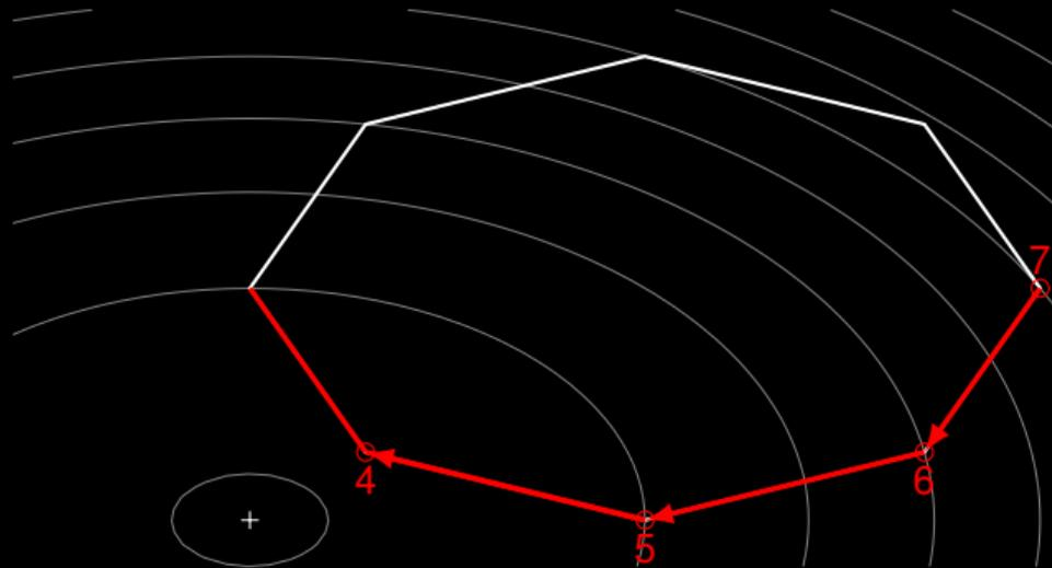
**Figure 26:** Illustration of active set method with two decision variables and initialised with two active constraints. The feasible region is within the octagon, the contour lines indicate the level sets of the cost function, the plus indicates the unconstrained optimum and the filled circle indicates the optimal solution.
