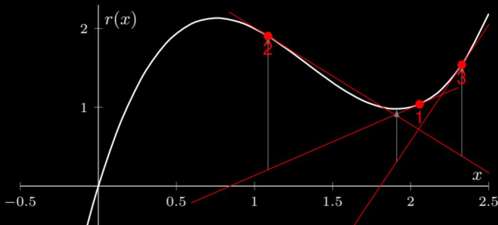
**Figure 23:** The Newton method converges to a stationary point where derivative is zero. The method loses a search direction and is not able to solve the problem.
