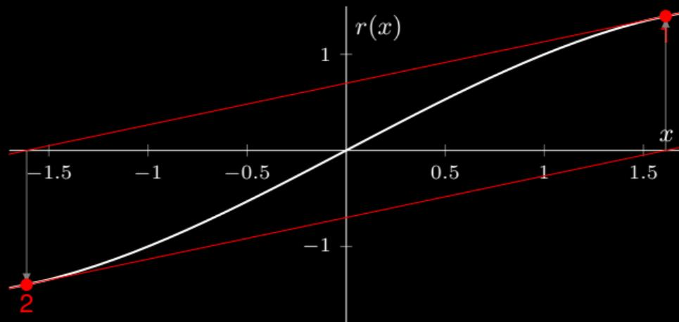
Figure 21: Failure of the Newton method to converge when using a full step size.
