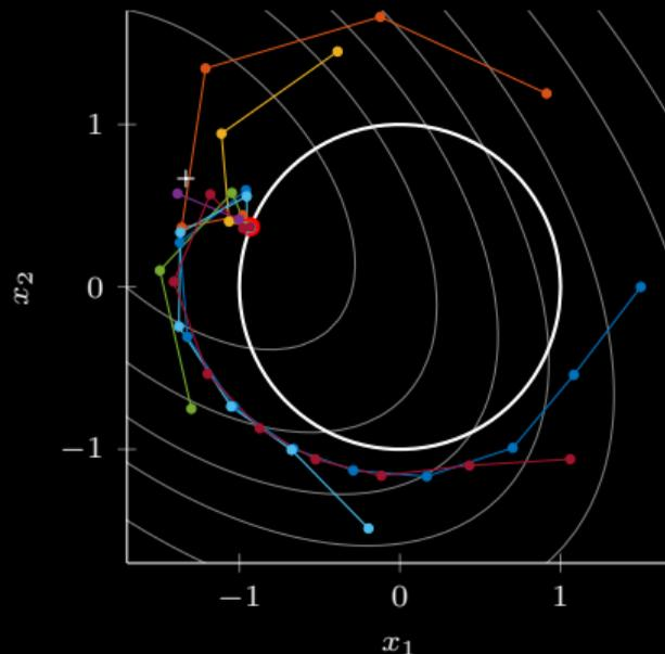
**Figure 24:** An illustration of the Newton method on an equality constrained problem. It can be seen that different initialisations require different number of steps until convergence.
