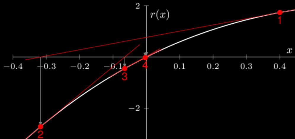
Figure 20: An illustration of the Newton method using a full step size. The method converges in about 4–6 steps, with a roughly quadratic convergence rate.
