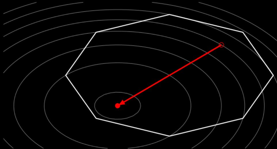
**Figure 29:** Illustration of active set method with two decision variables and initialised with inactive constraints. The feasible region is within the octagon, the contour lines indicate the level sets of the cost function, the plus indicates the unconstrained optimum and the filled circle indicates the optimal solution.
