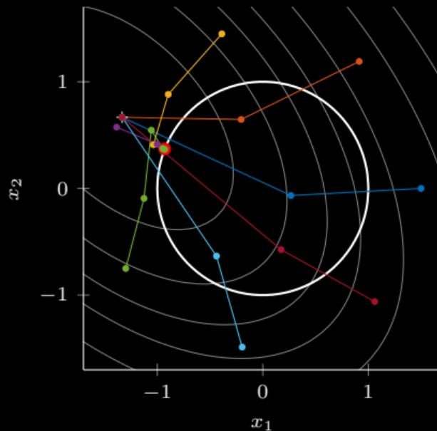
Figure 31: An illustration of the Newton method on an inequality constrained problem.
