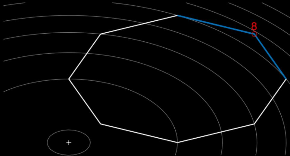
**Figure 27:** Illustration of active set method with two decision variables and initialised with two active constraints. The feasible region is within the octagon, the contour lines indicate the level sets of the cost function, the plus indicates the unconstrained optimum and the filled circle indicates the optimal solution.
