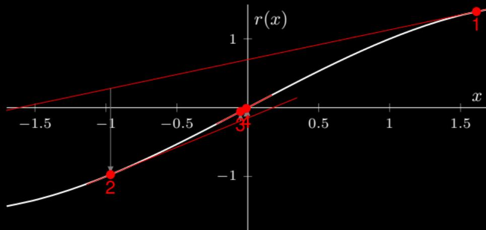
Figure 22: The Newton method using a reduced step size of 0.8. The method converges in about four steps.
