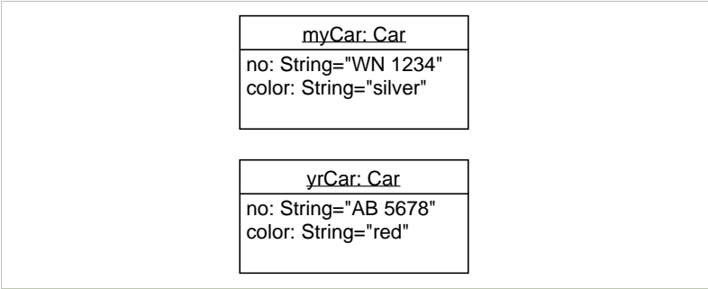
Figure A.1: An object diagram with two objects
