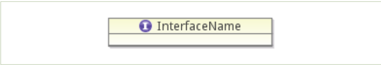
Figure A.4: EMF's syntax for interfaces
