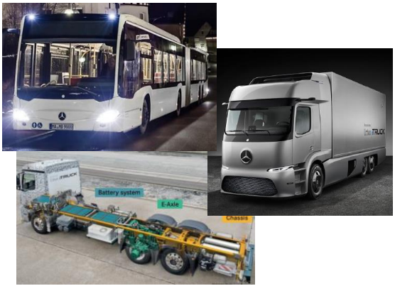
Daimler: The entire conventional drivetrain being replaced by a new electrically driven rear axle with electric motors
