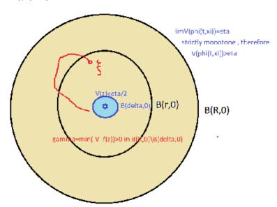
2) Now we continue proving that  $\lim_{t\to\infty} V(\varphi(t,\xi) = 0$ . By conditions of the theorem  $\frac{d}{dt}V(\varphi(t,\xi) < 0$ , therefore  $V(\varphi(t,\xi))$  is a monotone strictly decreasing function of t bounded from below because  $V(x) \geq 0$  and must have a limit
