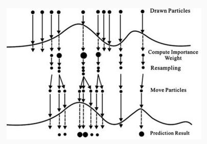
The next animation illustrates the concept of sequential importance sampling resampling with N=5 particles.
