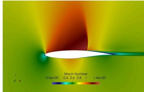
Figure 2: Mach number contours indicating shock wave pattern and flow separation over RAE 2822 airfoil.
