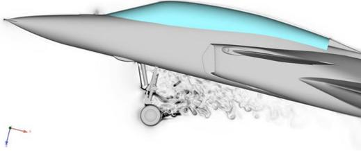
Figure 1: Density gradients of resolved turbulence behind nose landing gear. Used with permission by Saab.
