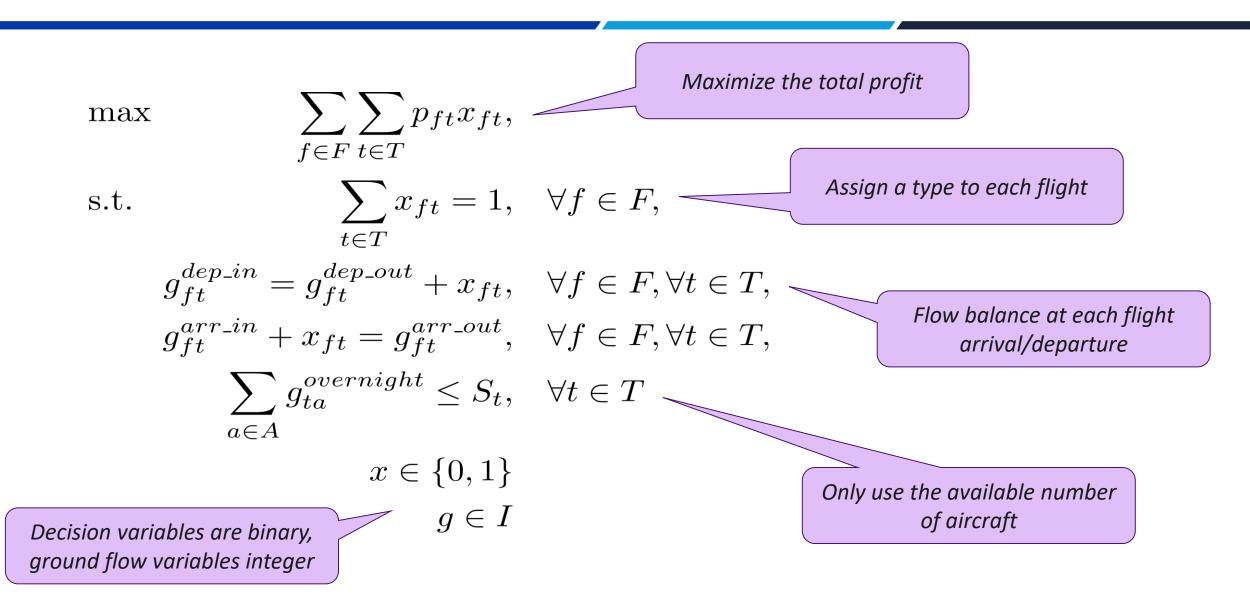
The presented model is a **multi-commodity network flow model** – one network flow model per aircraft type, connected by a few constraints.
