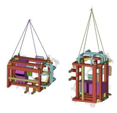
Verification of design compliance of SFT transportation skid and protection frame to DNV code 2.7-3
