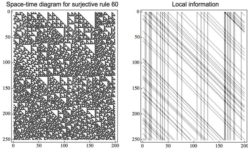
**Fig. 4.15** The space-time CA pattern for rule R60, and the corresponding information density picture. Here the information density  $I_{i,n}$  is derived analytically. A numerical estimate would not be computationally possible because of the linearly increasing correlation lengths.
