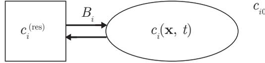
**Fig. 7.2** A schematic illustration of the open reaction-diffusion system, with concentrations  $c_i(\mathbf{x}, t)$ . There is a diffusion-controlled flow  $B_i$ , between the system and a reservoir, in which the concentrations,  $c_i^{(\text{res})}$ , are assumed to be kept constant. As a reference, the environment is assumed to be in homogenous equilibrium characterised by concentrations  $c_{i0}$ .
