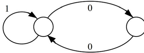
**Fig. 3.7** Finite automaton generating sequences of 0's and 1's in which 1's are always separated by an even number of 0's.
