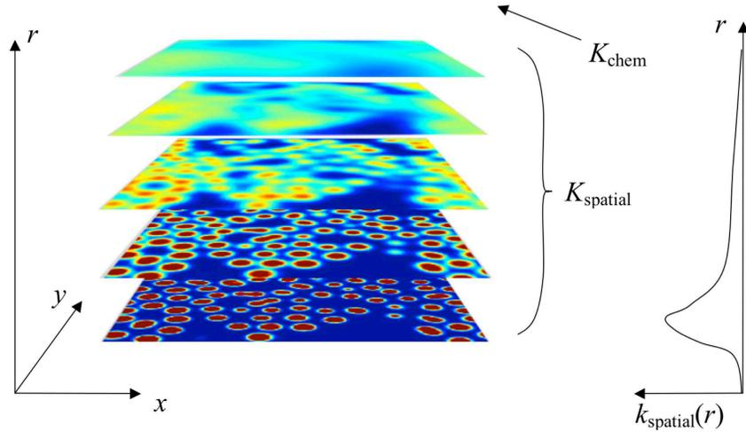
**Fig. 7.1** An illustration of a two-dimensional chemical pattern at different levels of resolution  $r$ , along with a schematic illustration on how the spatial information may be decomposed between different length scales. The chemical information can be detected regardless of how bad the resolution is and it is therefore located at infinite  $r$ .
