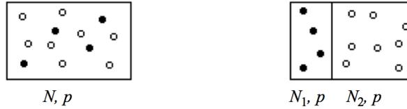
**Fig. 5.2** The two gases are mixed in the container to the left, but to the right they are separated by a wall so that the pressure is equal in the two parts.
