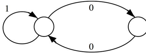
**Fig. 3.10** Example of hidden Markov model, represented by finite automaton generating sequences of 0's and 1's in which 1's are always separated by an even number of 0's. The probability for the arcs leaving the left node are both 1/2.
