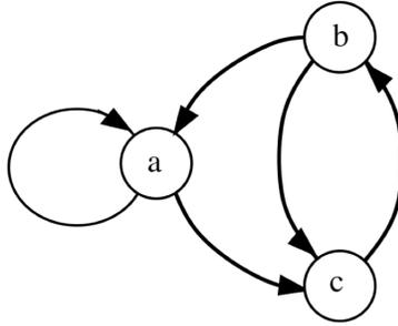
**Fig. 3.3** Example of finite state automaton representing a Markov process.
