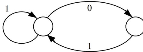
**Fig. 3.6** The finite automaton generates an infinite sequence of "0" and "1" by following the arcs between the nodes in the graph. When there are two arcs leaving a node, one is chosen randomly with equal probabilities for both choices.
