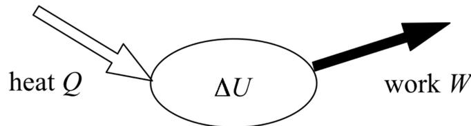
**Fig. 5.1** The first law of thermodynamics states that energy is a conserved quantity. The change in internal energy  $U$  is determined by the net energy difference resulting from the inflow of heat  $Q$  and work extracted from the system  $W$ .
