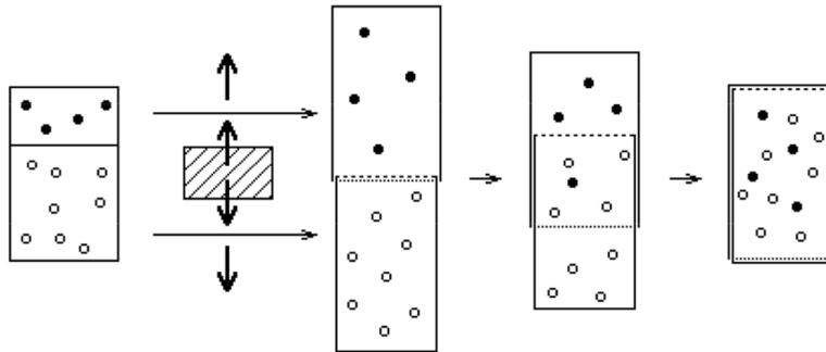
**Fig. 5.3** The two gases are mixed reversibly by an isothermal expansion in which work is done, followed by a fully reversible mixing without any energy transfer.
