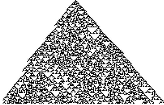
**Fig. 4.4** The difference pattern resulting from the time evolution of CA rule R22 starting from two different states, initially differing only by the state in one cell.
