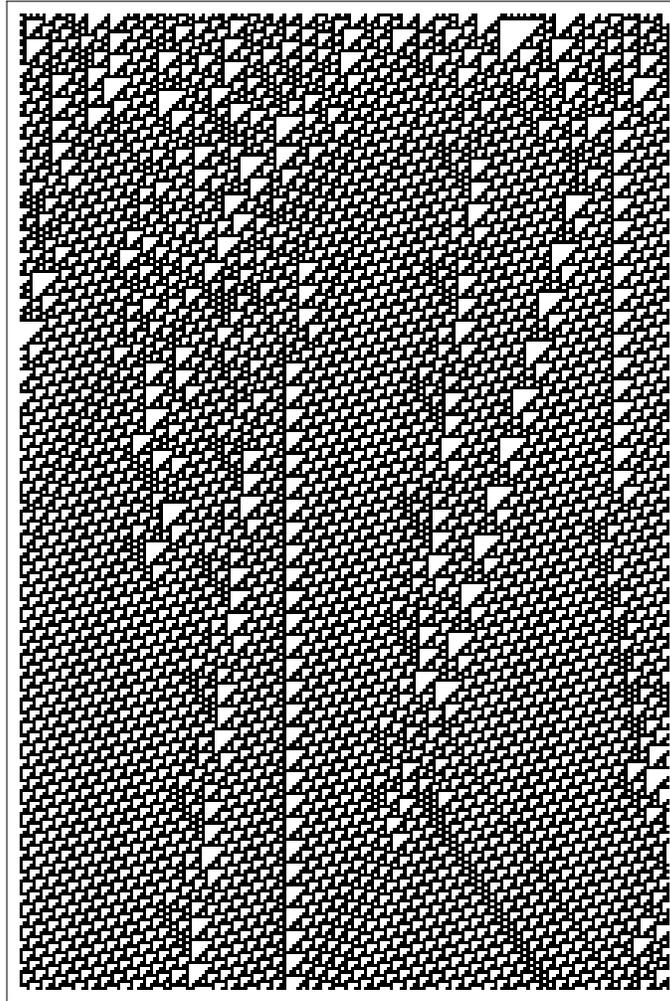
**Fig. 4.2** The time evolution of CA rule R110 starting with an "random" initial state (in the top row) shows how a periodic background pattern is built up at the same time as complex structures propagate and interact. This is a good example of the complexity that simple CA rules may exhibit.
