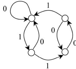
**Fig. 4.13** The most compact FSA representation of the CA state characteristics for time  $t + 1$ , when elementary CA rule R86 is applied to a CA state characterised by the FSA in Figure 4.10a at time  $t$ .
