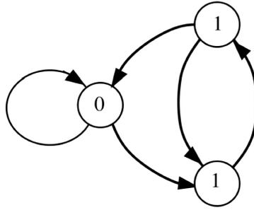
**Fig. 3.5** Example of finite state automaton representing a Hidden Markov model based on the Markov process of Figure 3.3.
