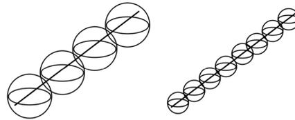
**Fig. 6.3** The number of spheres with radius  $r$  that are needed to cover a curve is proportional to  $r^{-D}$ , where  $D$  is the fractal dimension of the curve. In the figure, the number of spheres doubles as the radius is reduced to half the original, implying a curve dimension  $D = 1$ .
