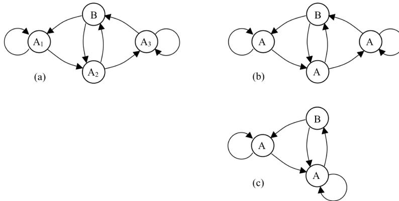
**Fig. 8.4** (a) The finite state automaton corresponding to the symbolic dynamics of the generating partition  $(A_1, A_2, A_3, B)$ . (b) The hidden Markov model corresponding to the symbolic dynamics of the non-generating partition  $(A, B)$  of Fig. (8.3), and (c) an equivalent representation of the hidden Markov model.
