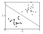
Line corresponding to  $P(t_{\text{new}} = 1 | \mathbf{x}_{\text{new}}, \widehat{\mathbf{w}}) = 0.5$ .
